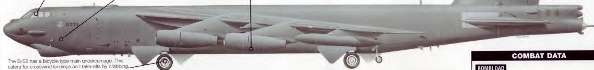
The B-52's wings can flex several metres up and down. Outriggers under the wingtips stop them from hitting the runway when carrying a full load of fuel and weaponry.
